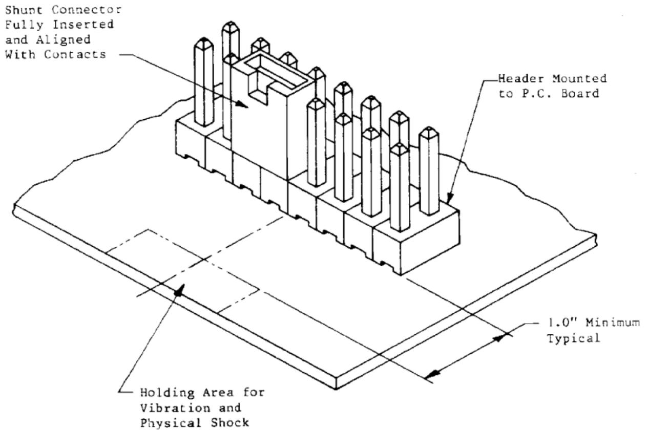
Holding Area for Vibration and Physical Shock
