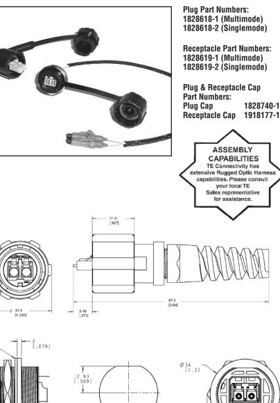
RECOMMENDED PANEL CUT-OUT MAX PANEL THICKNESS 3.2mm
